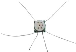
Prefabricated rat headmounts use fittings mounted on a 9X9 millimeter board with EEG or EMG electrode wires attached. An additional two-pin electrode is used for 4 EEG configurations.
