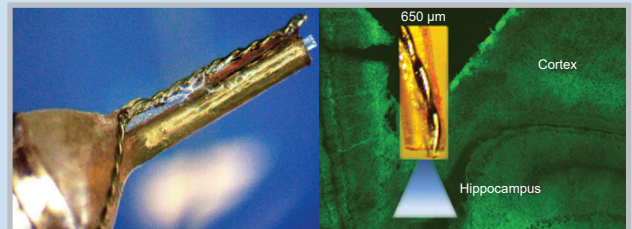
Histology slice showing the brain region near the implanted cannula and depth electrode. The blue shading shows the estimated LED light penetration from the 200 \mu\text{m} tip. Green coloring indicates channelrhodopsin expression in tissue.
